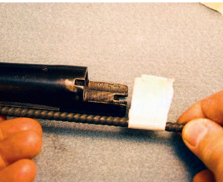
Reid says to position a marker flag on the Flex-Hone shaft at the breech end of the barrel so that the Flex-Hone does not pass over barrel ports or a screw-in choke tube.
