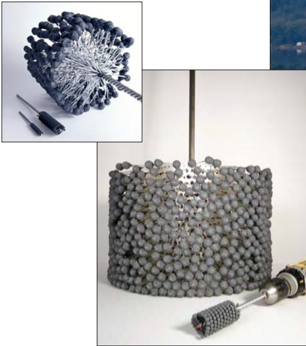
The photos to the left are some examples of Flex Hones – flexible, ball-style hones – that are successfully being used to pulverize nuclear waste.
